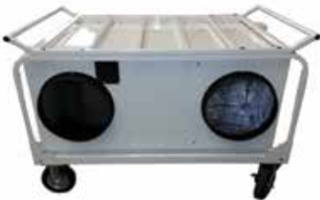
DI-100IFH Propane Indirect BTU/H: 100,000 CFM: 1850 Electrical: 115V/1PH/60Hz Power Draw: RLA 7.9 (985 Watts) Dimensions: 54.25" x 34.25" x 37.5" Weight: 363lbs
