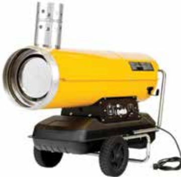
BV110E Multi-Fuel Indirect BTU/H: 112,800 CFM: 1060 Electrical: 115V/1PH/60Hz Amp Draw: 2.3 Dimensions: 48" x 26" x 40" Weight: 134.2lbs
